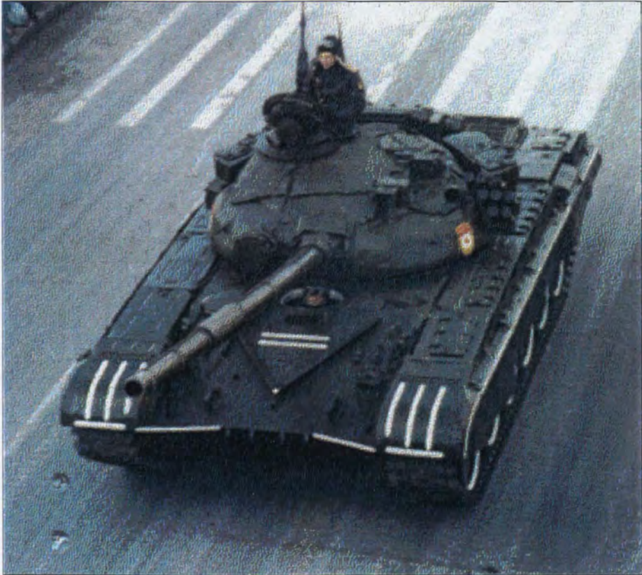
60 km/h, 1x125 mm 2A46 gun, 1x7,62 mm machinegun, 1x12,7 mm NSVT
