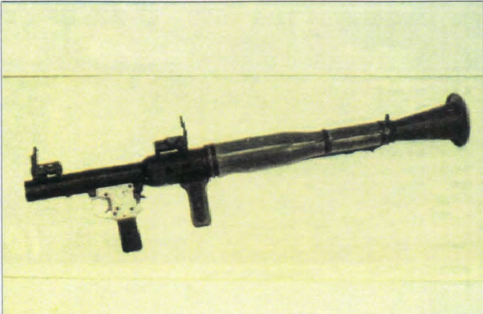
40 mm tube, 85 mm grenade, Range 500 m (depending on munition type)
