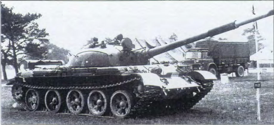
50 km/h, 1x115 mm Gun, 1x12,7 mm tl , 1x7,62 mm machinegun
