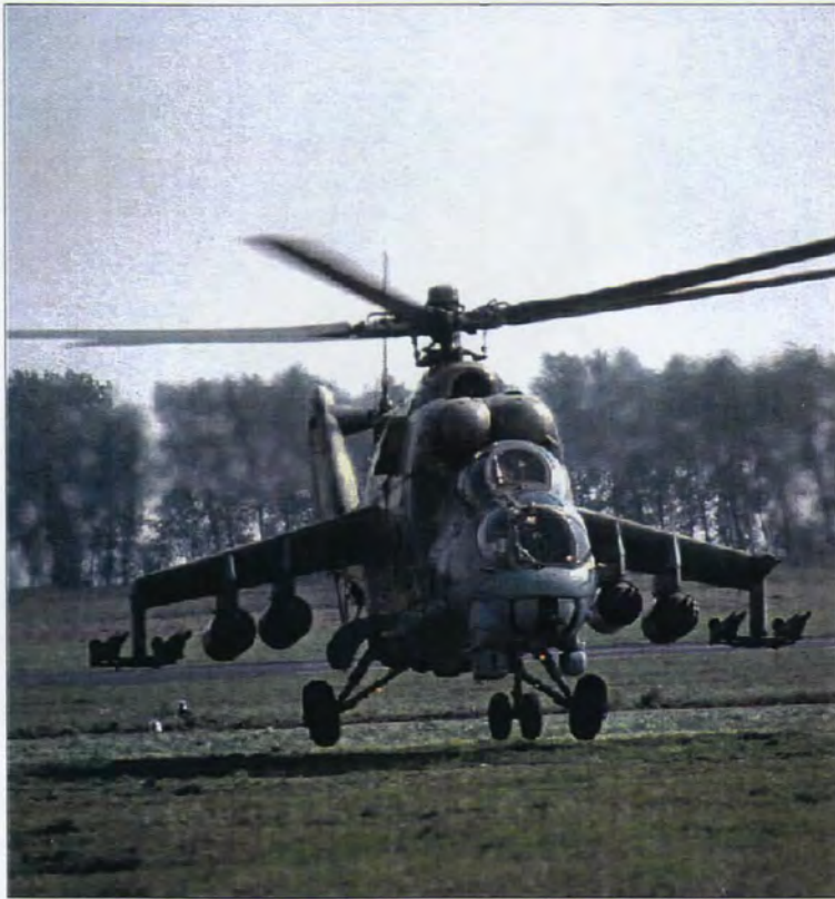
1x 4-barrel JakB 12,7 mm Gatlinggun, 4 S-80 rocket pods, AT-2 Swatter or AT-6 Spiral
