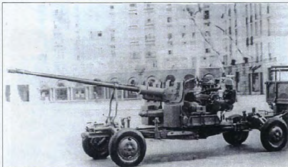
57 mm Anti-Aircraftgun, Range 12000 m
