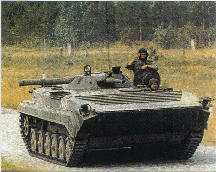
65 km/h, 1x73 mm gun, 2x7,62 mm machinegun, AT-3 Sagger missile
