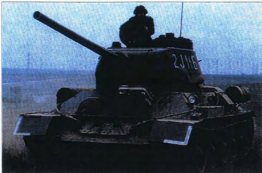
55km/h, 1x85mm gun, 7,62mm machinegun
