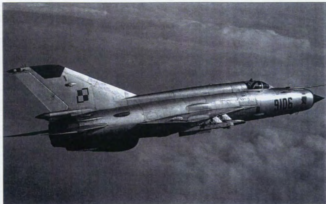
twin barrel 23 mm Gsh-23L gun, 4 underwing pylons for AA/AS missiles
